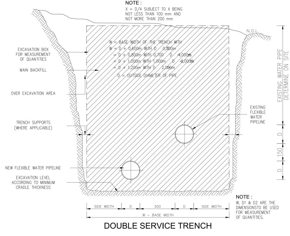
MEASUREMENT OF EXCAVATION SCALE 1:10
